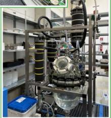
A demonstration unit for the new DAC process was set up at Axiom. The unit is able to capture a stream of 1 kg/h of atmospheric  $\mathrm{CO}_2$  and to provide it in the concentrated and pressurised state as feedstock for fuel syntheses. The last project year is dedicated to the experimental operation and evaluation of the DAC process.
